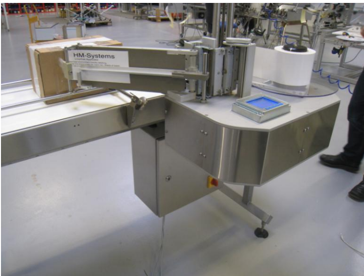
HM Linerfree Systems® MKII – An intelligent linerless print & apply system for e.g. box labelling eliminating backing paper, doubling up-time and reducing CO2 emissions
